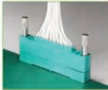
MB to I/O-C Discrete Wires to PCB
